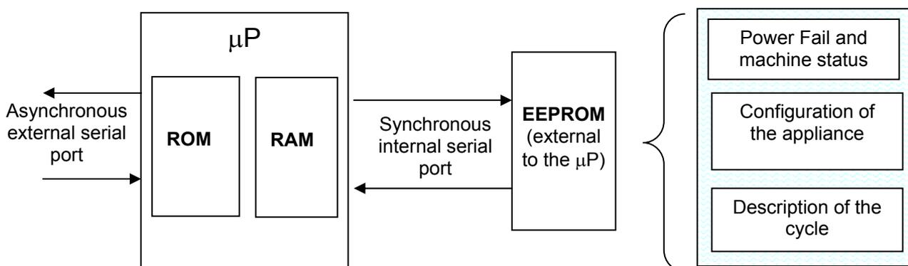
The main circuit board features an EEPROM memory (external to the microprocessor) which stores in memory data relative to the configuration, description of the cycle, cycle status in case of a power failure, and any alarm conditions.
