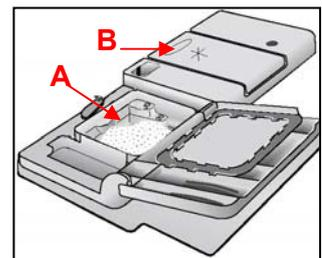
The coil of the detergent dispenser (DD) is powered by the circuit board via triac TY5 (connector D7) at certain points during the cycle, thus ensuring correct dosage.
