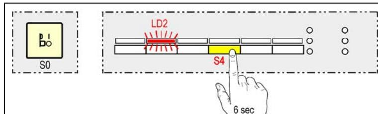
Until a cycle has actually started, the settings selected can be modified at any time by pressing the appropriate buttons. If the door has been closed, proceed as follows to modify the programme:
