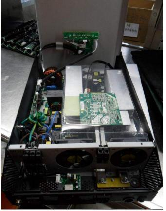
Remove the LCD and LED panel cables. There is the glue on the LCD cable connector, you can use a needle-nosepliers remove it slightly. Without cables on the top cover, you can place the top cover on the side.
