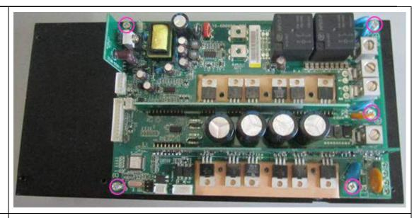
Take off the charger board. Until now the finish the SCC board disassembly.
