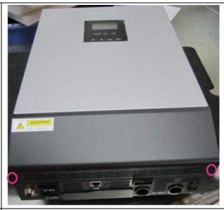
Remove the nuts of the battery connector.
