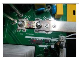
The U9 is 11-004003-00G (IC PWM CNTL ON/SG3525ANG DIP-16)
