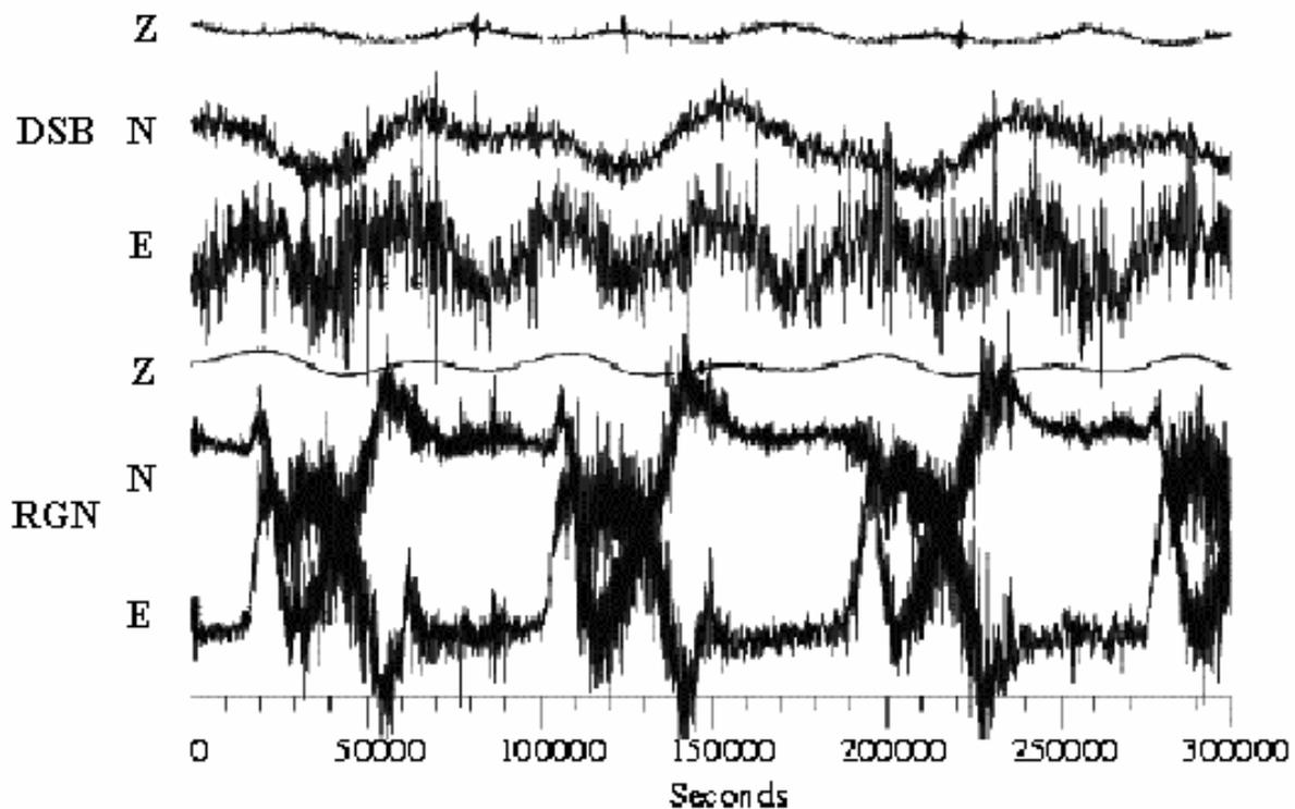
**Fig. 7.57** Comparison of two surface vaults in moderate climate on rock and in sediments. At DSB (Dublin, Ireland), a small surface bunker was built in an old granite quarry. At RGN (Rügen Island, Germany), an old one-room military bunker with a thin (< 1m) soil cover on top is used. Both sites host STS2 seismometers with GEOFON shielding.
