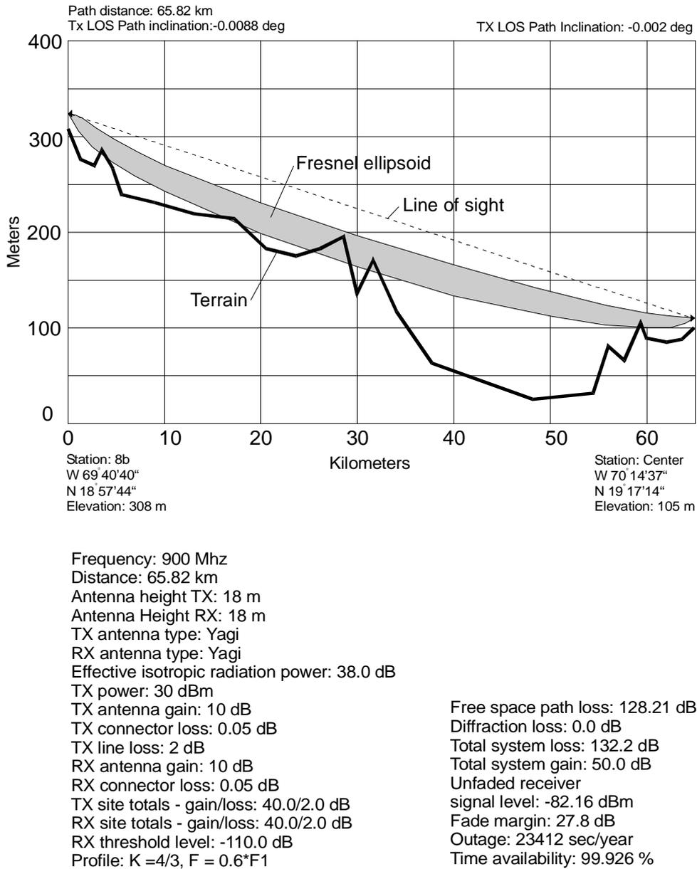
**Fig. 7.38** Result of an RF link calculation with input parameters on the left and output parameters on the right.
