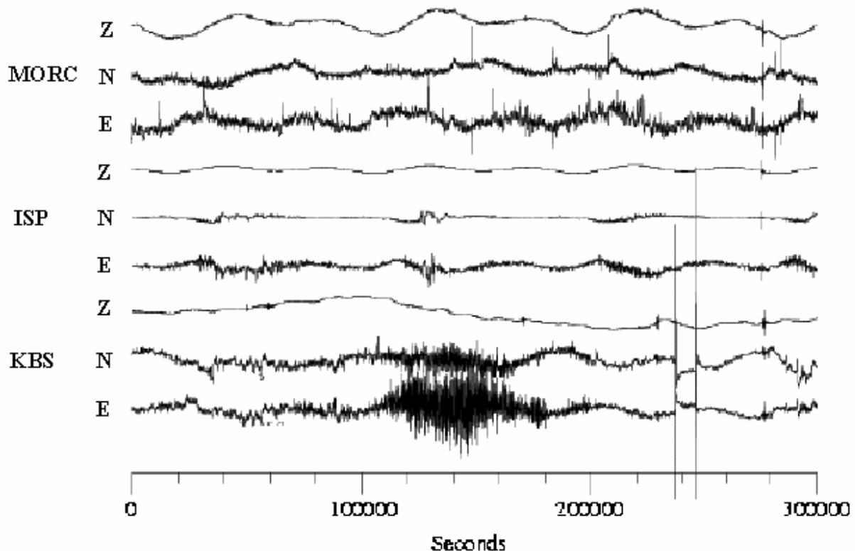
**Fig. 7.54** Comparison of three 3-component VLP records in shallow vaults (4 - 5 m). At MORC (Moravsky Beroun, Czech Republic) an STS2 is installed in a 1 m wide borehole in hard rock; in ISP (Isparta, Turkey) and KBS (Ny Alesund, Spitsbergen) sets of STS1/VBB are installed in underground bunker vaults in limestone and weathered rock (permafrost), respectively.
