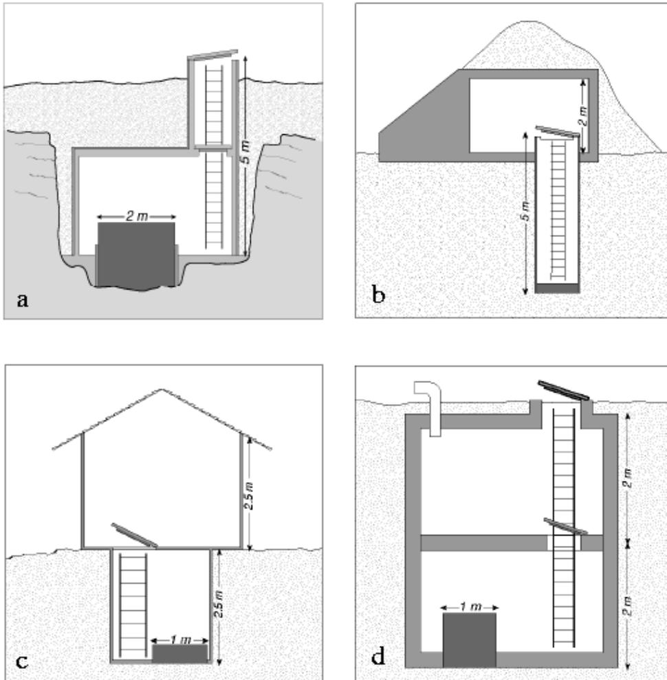
**Fig. 7.55** a) Underground bunker vault construction for the installation of a set of STS1/VBB (remote recording); b) "wide & shallow borehole" vault construction for the installation of an STS2; c) and d) simple bunker vault construction schemes for an STS2. The vault constructions b - d allow onsite data recording thanks to the existence of a separate recording room.
