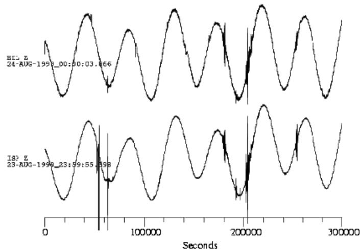
**Fig. 7.49** Tidal recordings of STS1/VBB and STS2 do not differ very much when properly installed in a comparable environment. The two traces were recorded in the Eastern Mediterranean in buried vaults in limestone. At the station EIL (Eilat, Israel) an STS2 with additional GEOFON shielding and at ISP (Isparta, Turkey) a set of STS1/VBB are installed.
