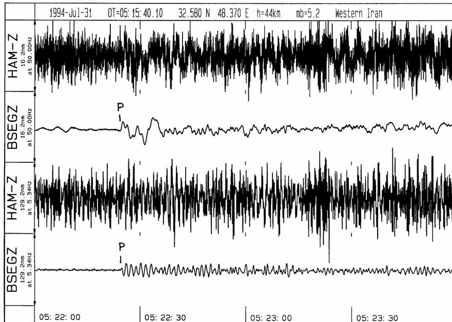
**Fig. 7.35** Z-component records of an earthquake in Iran (distance about 3800 km) at HAM and BSEG. Upper two traces: unfiltered broadband records; lower two traces: band-pass filtered with  $f = 0.5$ -5 Hz (from Bormann et al., 1997).
