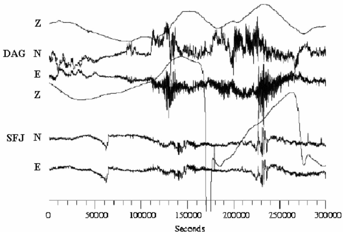
**Fig. 7.58** VLP records obtained at two surface vaults on Greenland. At DAG (Danmarkshavn, NE Greenland) a STS2 in GEOFON shielding is installed in a wooden hut on weathered rock close to the sea shore. At SFJ (Sondre Stromfjord, SW Greenland) a set of STS1/VBB is located in a container-like building on top of a mountain. In both cases the geology is weathered rock in a permafrost environment.
