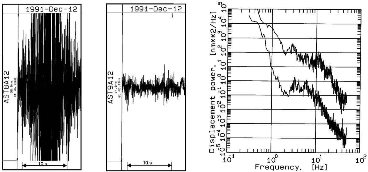
**Fig. 7. 20** Comparison of seismic records and related noise spectra made at the time of passing of a heavy truck: Left: record near the road embankment; middle: record made about 1 km away from the road in the countryside (middle); right: noise power density spectra. Underground: wet Alluvial coastal plain deposits. (Note that the noise amplitudes in the left panel have been reproduced with only 40 % of the magnification in the central panel).
