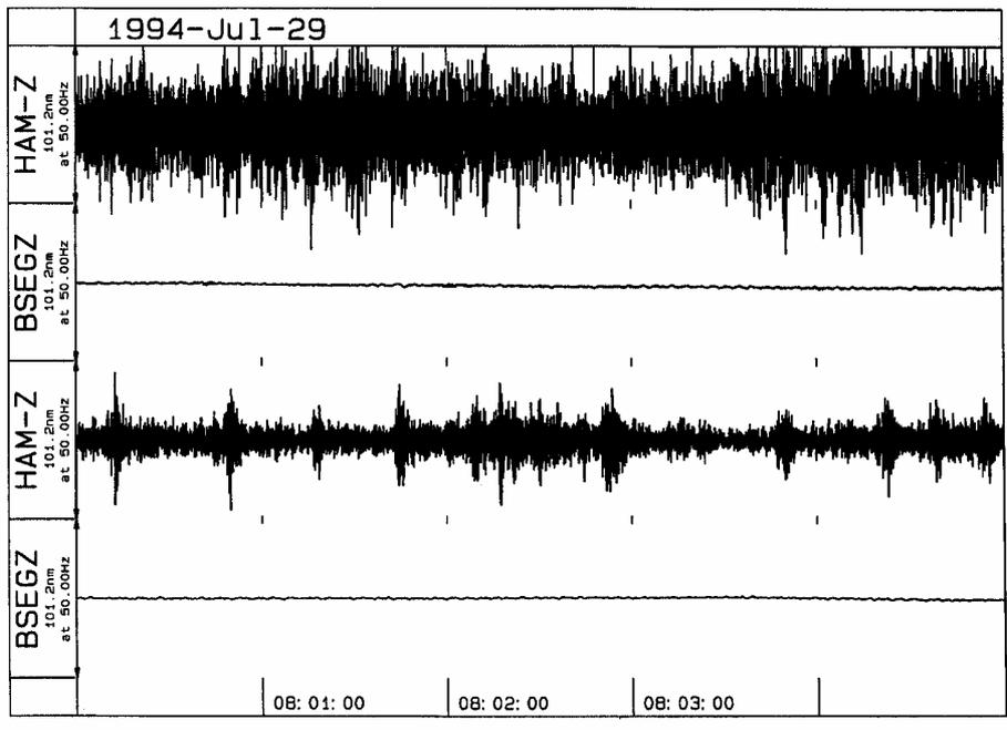
**Fig. 7.33** Five minutes of unfiltered Z-component broadband records at HAM and BSEG on July 29, 1994 at 8:00 UT in the morning (upper two traces) and after midnight (lower two traces) (from Bormann et al., 1997).
