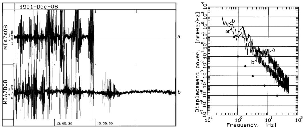
**Fig. 7.18** Noise records (left) and related power spectra (right) at a remote low-noise hard rock site in NW Iran. The large, impulse-like amplitudes in the first part of the record are due to the movement of team members near to the sensors. Note the much lower noise (dots in the spectrum) after they were asked to "sit down and be quiet".
