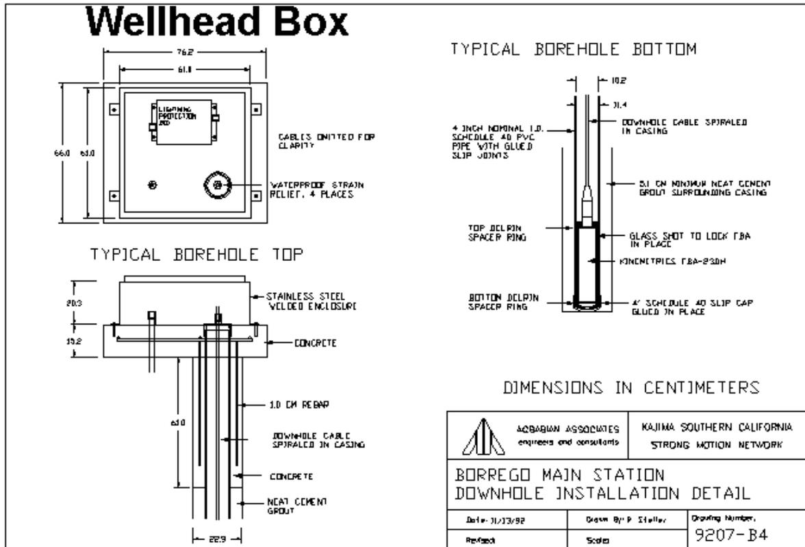
**Fig.7.62** Sketch of borehole strong-motion accelerometer installation details.
