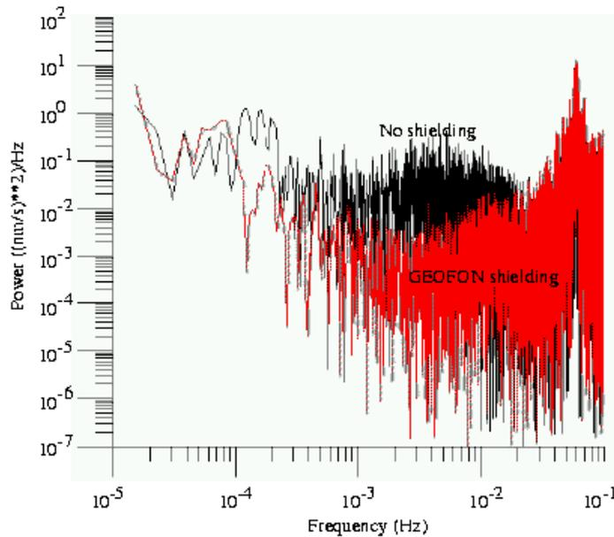
**Fig. 7.51** VLP noise reduction achieved by using the simpler version of the GEOFON shielding method (no additional polystyrol box and beads ). The relative noise power spectra of the vertical component of two STS2s positioned side-by-side are shown. No instrument correction has been applied. The black spectrum is from the unshielded STS2, the red spectrum from the shielded one.
