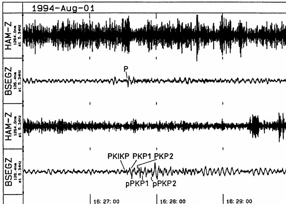
**Fig. 7.37** Short-period band-pass filtered Z-component recordings ( $f = 0.5 - 5\text{Hz}$ ) at HAM and BSEG. Upper two traces: P-wave onset of a Kurile Islands earthquake on 01.08.94 ( $D = 76.2^\circ$  to HAM,  $m_b = 5.0$ ); lower two traces: PKP-wave group from an earthquake in the Tonga Islands on 30.07.94 ( $D = 150.1^\circ$  to HAM,  $m_b = 5.0$ ) (from Bormann et al., 1997).
