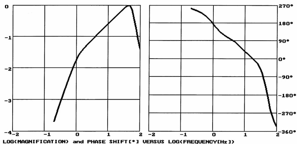
**Fig. 7.11** Amplitude and phase response curves for the seismometer-recorder combination SS-1/SSR-1 as used in field measurements in NW Iran (see Figs. 7.12 to 7.21). The response is proportional to velocity between about 1 and 50 Hz.
