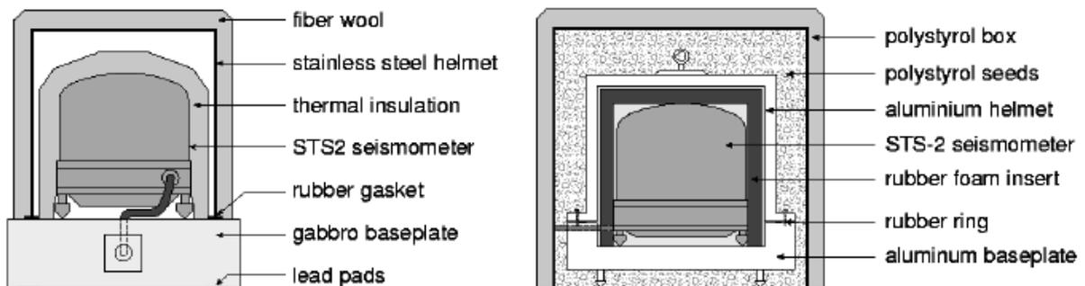
**Fig. 7.50** GRSN (a) (after Wielandt, 2000) and GEOFON type (b) shielding for the STS2.
