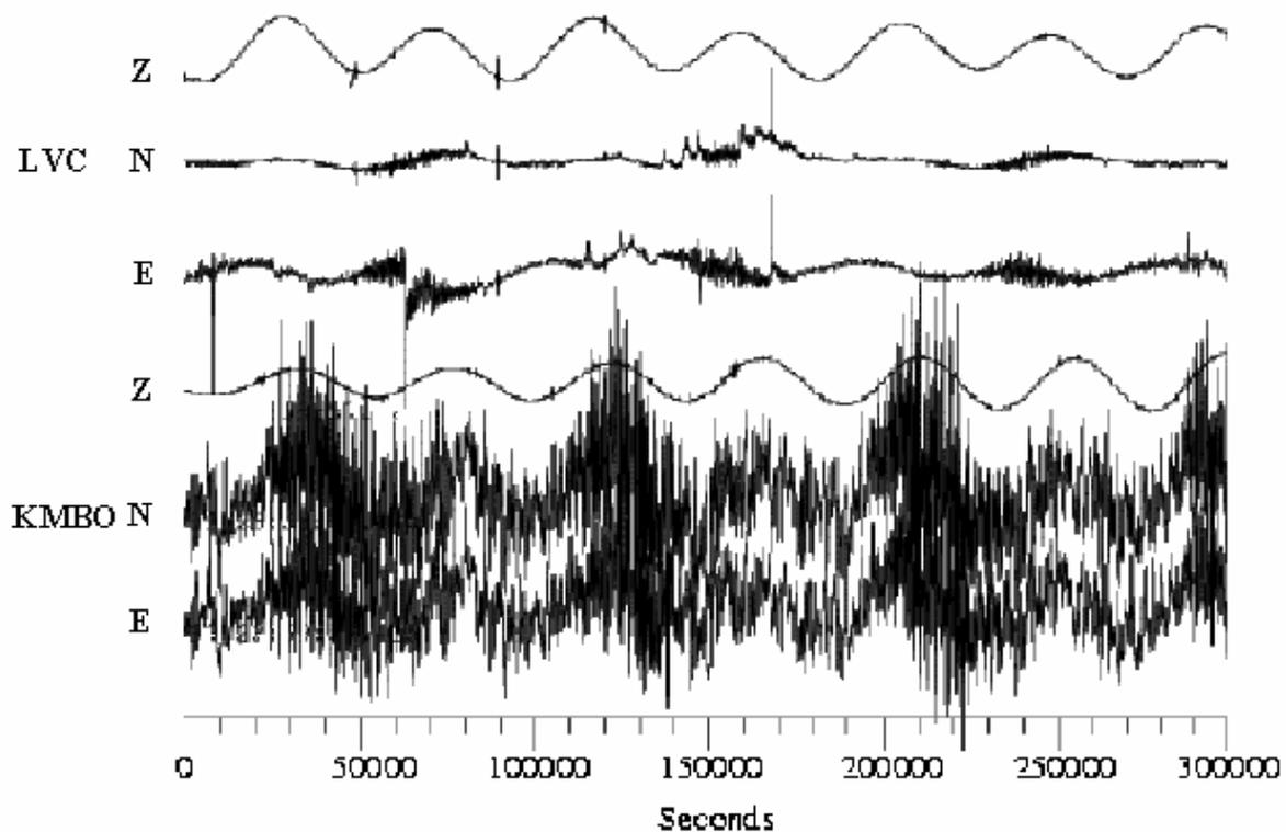
**Fig. 7.53** Comparison of two 3-component STS1 VLP traces recorded in identical tunnel constructions but in different geological and climatological environments. LVC (Limon Verde, Chile) is built in hard basaltic rock in a full desert environment, KMBO (Kilima Mbogo, Kenya) is placed in rather soft volcanic conglomerate influenced mostly by a humid tropical environment. Day-to-night temperature gradients are high in both cases.
