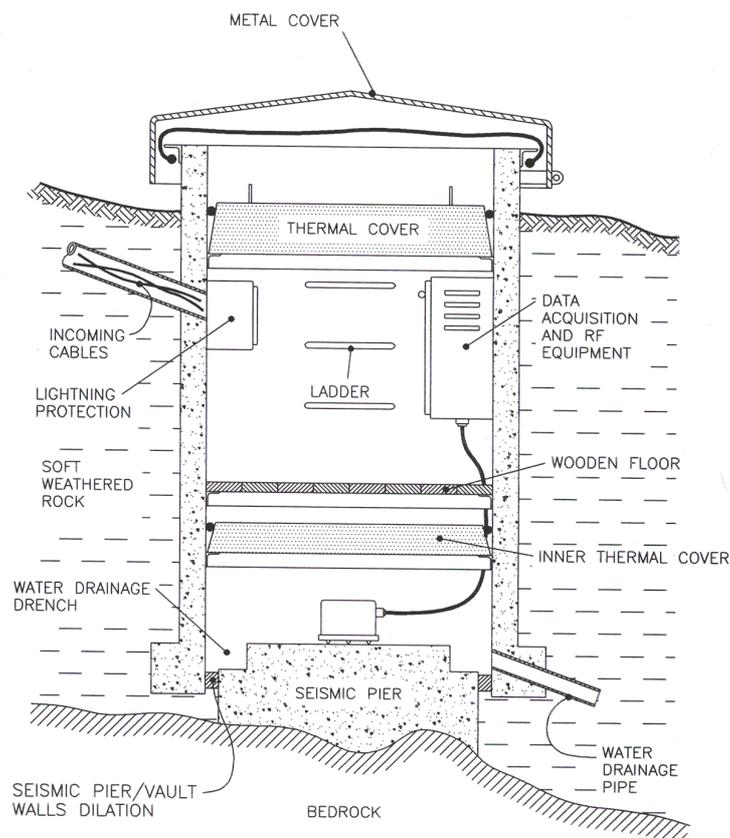
**Fig. 7.44** Example of a BB or VBB seismic vault with a separate compartment for sensors and double thermal cover. Usually, the sensor itself is additionally isolated (see Fig. 7.50). A thermal isolation box is usually put around the sensors to additionally insulate them.
