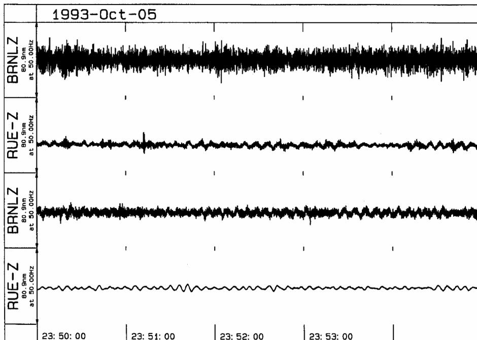
**Fig. 7.30** Unfiltered Z-component broadband records of seismic noise with identical resolution at BRNL and RUE. Upper traces: 11:50 - 11:55 UT; lower traces: 23:50 to 23:55 UT (from Bormann et al., 1997).
