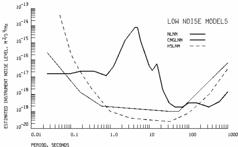
**Fig. 7.60** Low-noise models for the KS-54000 (KSLNM) and the CMG-3TB (CMGLNM) sensor system self-noise relative to Peterson's (1993) new low-noise model (NLNM) for background Earth's motion.
