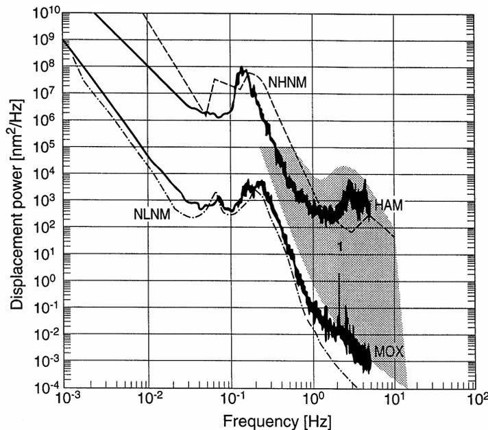
**Fig. 7.27** Spectra for the noisiest day observed at HAM (January 13) and the quietest day at MOX (May 23) during 1993. The NHNM and NLNM according to Peterson (1993) are shown for comparison. The shaded area (1) covers the range of short-period noise power calculated by Henger (1995) for all GRSN stations on March 1, 1994 (modified from Bormann et al., 1997).
