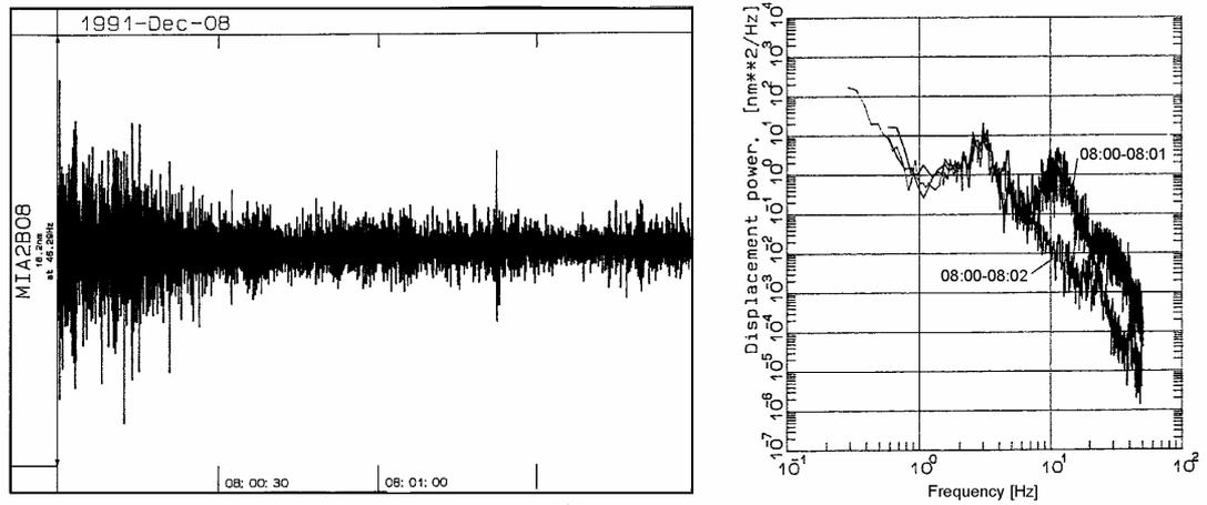
**Fig.7.17** Noise record and related spectra for the first minute (transient) and second minute (background noise). The transient is due to a truck passing by at several 100 m distance from the recording site.
