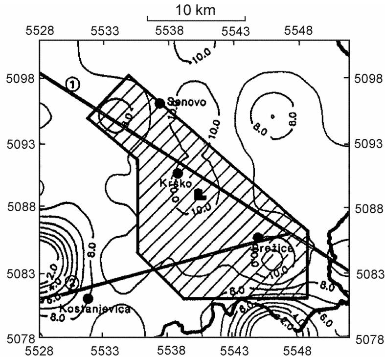
**Fig. 7.3** Final choice of the area to be studied in detail by the seismic network (hatched area). Also shown are the isolines of released log-seismic energy during the time-span of the catalogs (in J/km<sup>2</sup>).
