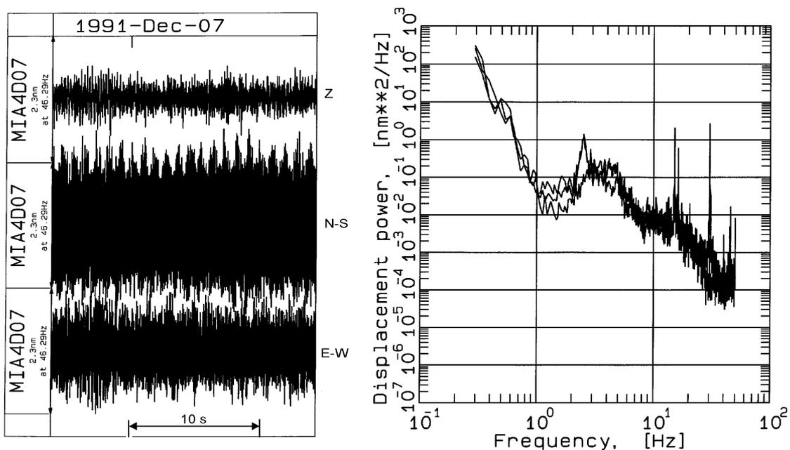
**Fig. 7.19** Noise records and related power spectra near to a transformer house and power line. Note the monochromatic spectral lines around 13, 30 and 50-60 Hz, either induced by the AC current frequency and its lower harmonics and/or caused by the vibration of the transformer.
