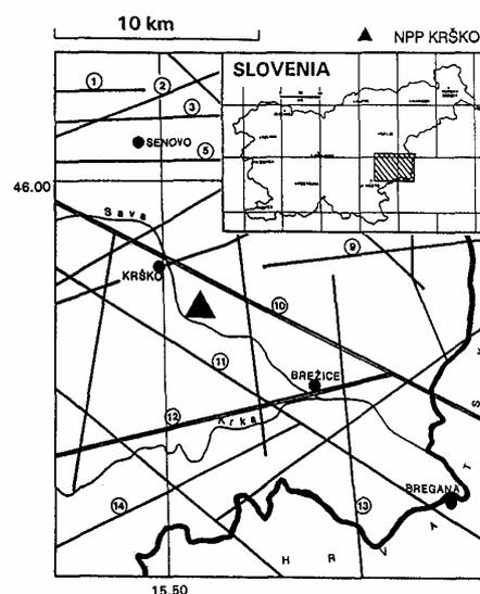
**Fig. 7.1** The broader region chosen for the network in Slovenia and the main geological faults in this area (9 - Artice fault, 10 - Brestanica fault, 11 - Sava fault, 12 - Podbocje fault, 13 - Brežice fault, 14 - Orehovec fault).
