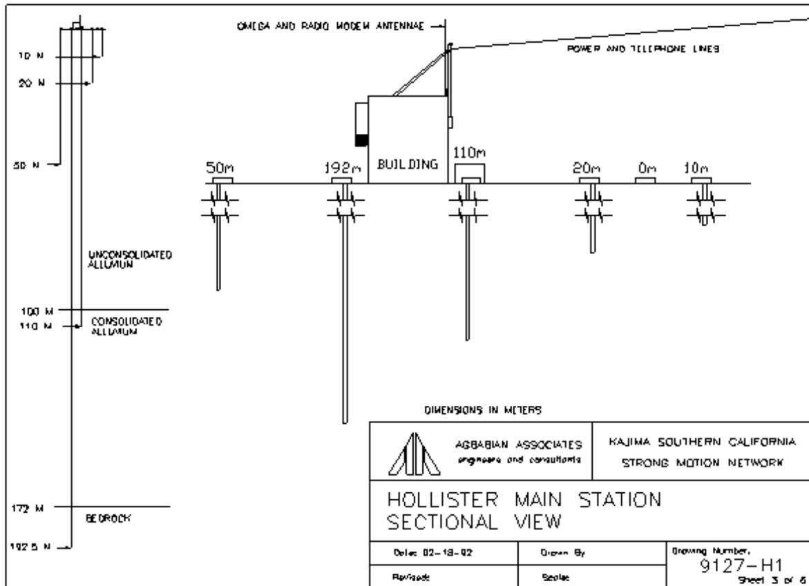
**Fig. 7.63** Sketch of a borehole strong-motion array.
