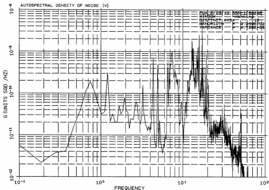
**Fig. 7.7** Typical seismic noise spectrum (ground velocity power density in  $\text{m}^2/\text{s}^2/\text{Hz}$ ) at a potential seismic station site showing man-made seismic noise generated by a nearby city and heavy machinery working in a 4 km distant quarry.
