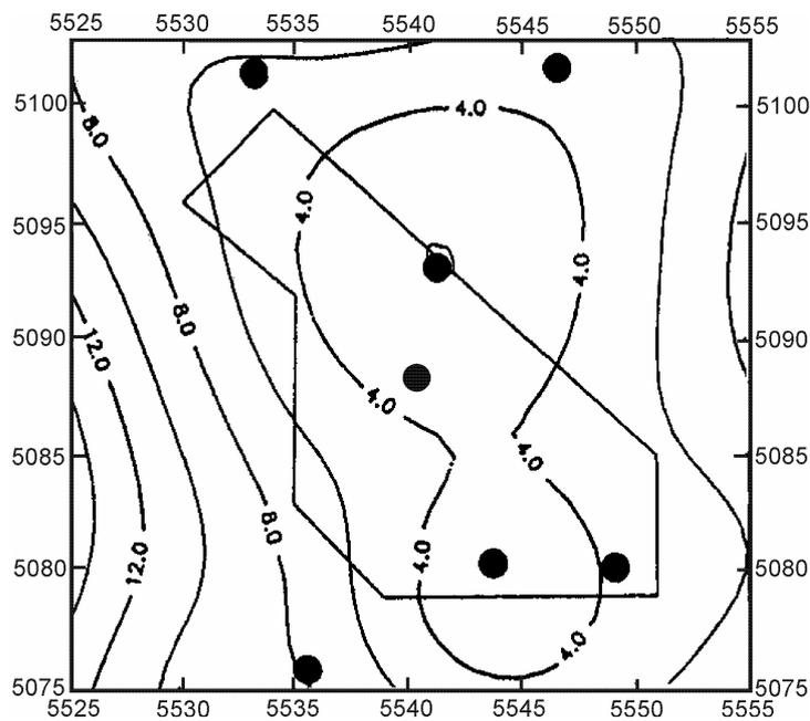
**Fig. 7.10** An example of computer modeling of network capability. Isolines of uncertainty of hypocenter determination in km ( $\pm 1$  standard deviation) are shown for the best of the alternative network layouts.
