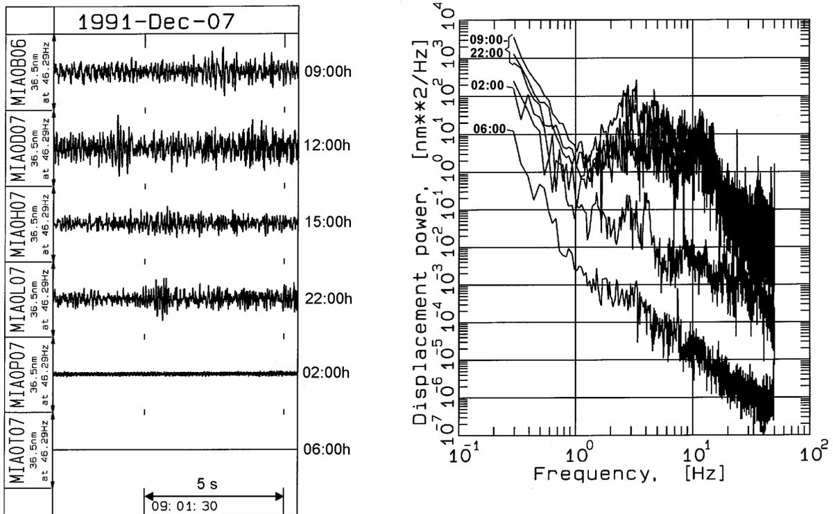
**Fig. 7.15** Comparison of relatively quiet sections of vertical component noise records (left; without strong transients) and related power spectra (right) at a reference site in a town in NW Iran. The measurements were made at different times of the day.
