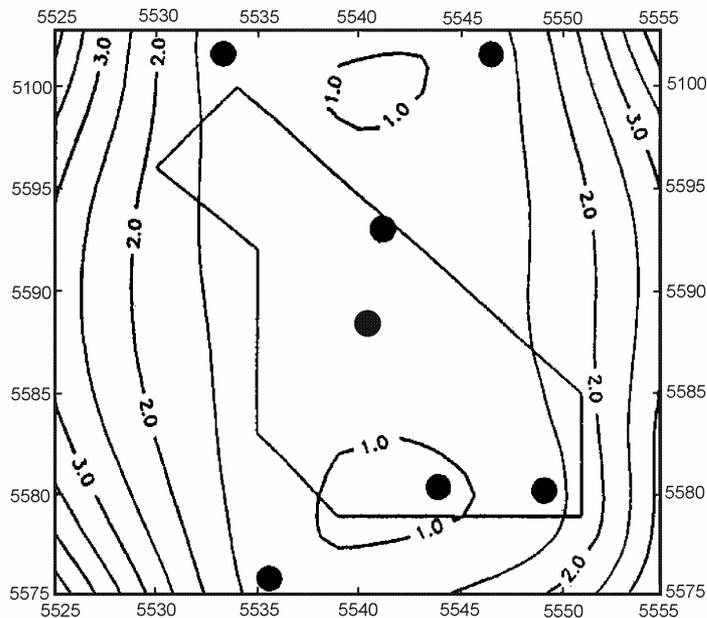
**Fig. 7.9** An example of computer modeling of network capabilities. Isolines of uncertainty of epicenter determination in km ( $\pm 1$  standard deviation) are shown for the best of the alternative network layouts.
