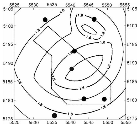
**Fig. 7.8** An example of computer modeling of network capabilities. Isolines of minimum magnitude of events detected at 5 seismic stations (from six in the network) with a signal-to-noise-ratio  $>20$  dB are shown for the best of the alternative network layouts.
