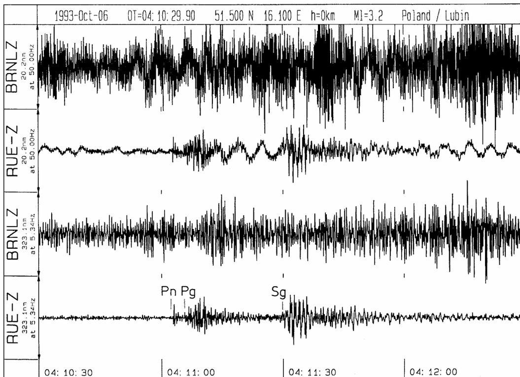
**Fig. 7.32** Unfiltered broadband (upper two traces) and band-pass filtered ( $f = 0.5 - 5$  Hz; lower two traces) Z-component records of a near seismic event in Poland at BRNL ( $D = 214$  km) and RUE ( $D = 191$  km) (from Bormann et al., 1997).
