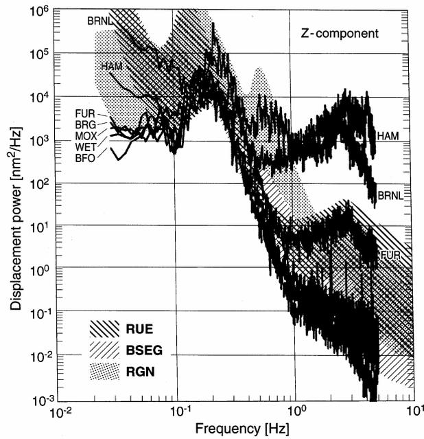
**Fig. 7.24** Displacement power density spectra at selected GRSN stations determined from noise records on the morning of April 13, 1993. For comparison the ranges of noise power observed at the new sites BSEG, RGN and RUE are given as shaded areas (from Bormann et al., 1997).
