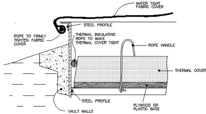
**Fig. 7.43** Detail of making a thermal cover effective by filling up the gaps between the cover and vault walls with insulation material and making the vault tight against dust, dirt, and rain during windy periods with a fabric cover.
