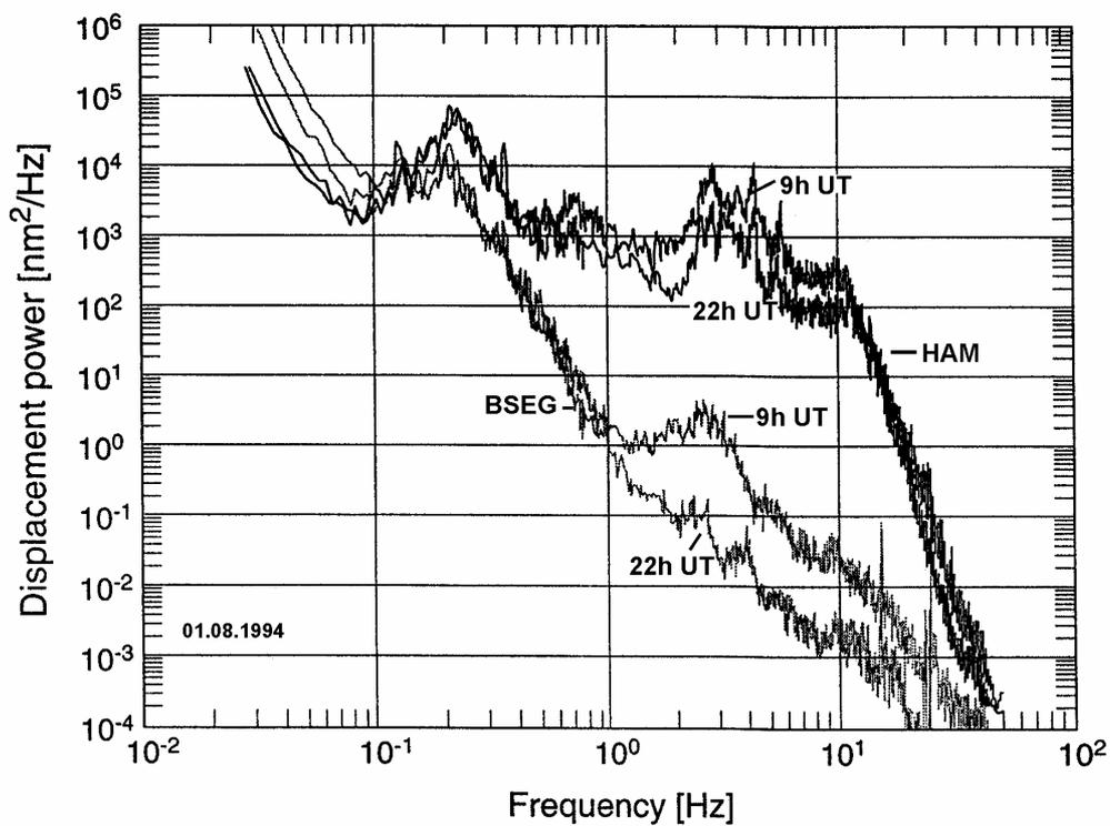
**Fig. 7.34** Noise power spectra at HAM (upper two curves) and BSEG (lower two curves) determined from Z-component records on August 1, 1994, around 9 h UT and 22 h UT, respectively (from Bormann et al., 1997).
