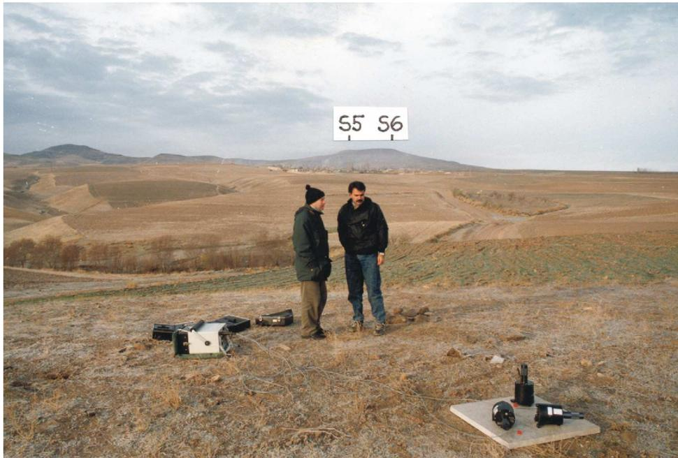
**Fig.7.13** Temporary three-component reference installation in NW Iran on a leveled marble plate placed on unconsolidated ground. Two other measurement points on the horizon using outcropping hard rock are marked. The noise at the latter sites was close to the NLNM.
