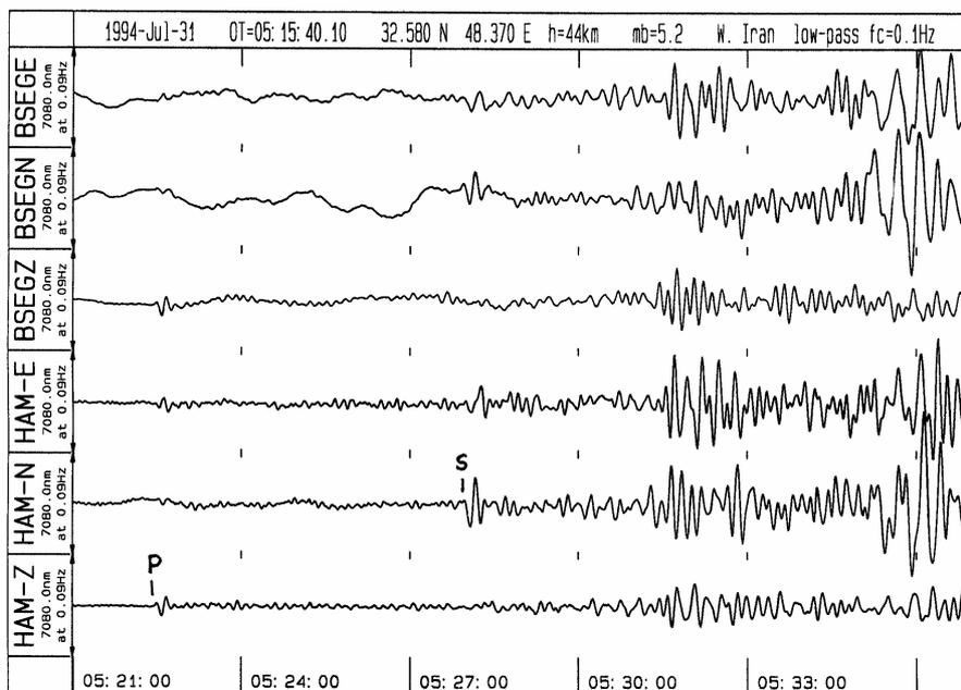
**Fig. 7.36** Low-pass filtered ( $f_c = 0.1$  Hz) long-period 3-component records at BSEG and HAM of the Iran earthquake (from Bormann et al., 1997).
