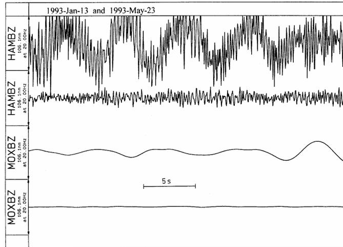
**Fig. 7.26** Comparison of record segments with largest (13 January) and lowest seismic background noise (23 May) observed in 1993 at stations HAM (upper two traces) and MOX (lower two traces) (from Bormann et al., 1997).
