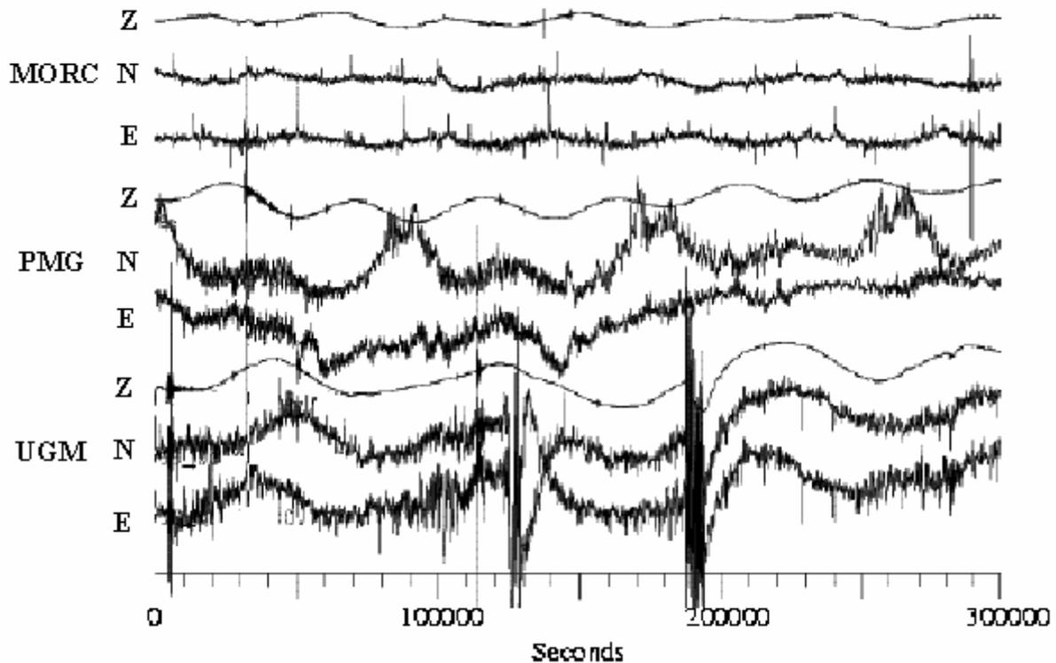
**Fig. 7.56** Comparison of three 3-component VLP records from shallow vaults in rock in different climates. Data from two sites close to the equator (Port Moresby, Papua New Guinea, PMG, and Wanagama, Indonesia, UGM) are shown together with data from MORC (same station as in Fig. 7.54).
